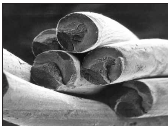
Fig. 12: Fatigue cracks starting at the points of contact of individual wires. The cracks became visible after destroying the strand in a pull test.
