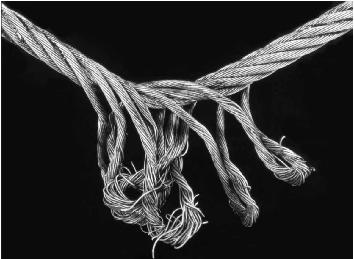
Fig. 107: This steel wire rope has been unlaid. In this state its outer strands are too long for the rope length. A sheave has accumulated the “superfluous” strand lengths to a point at the end of its travel.
