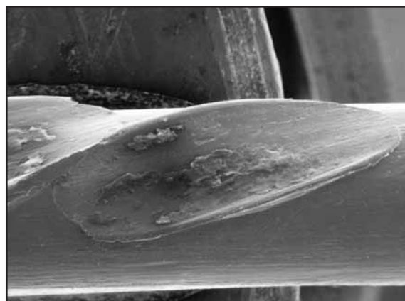
Fig. 94: The cross over marks between two strand layers are often the starting points for fatigue cracks inside the rope.
