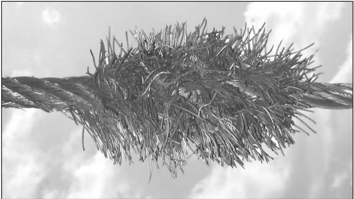
Fig. 61: Closing rope of a grab crane. All the outer wires had broken due to severe abrasion. The flared exit funnel of the grab has pushed all loose wire ends along the rope length to one location, creating this impressive hedgehog.
