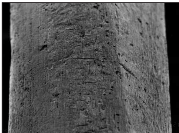
Fig. 13: Surface corrosion often initiates the formation of fatigue cracks.
