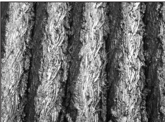
Fig. 136: Rope damage on a multi layer drum. It took one of the authors a considerable time to convince the user that...
