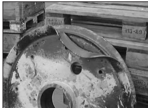
Fig. 123: Extreme wear on the flange will one day cause it to collapse. During inspection, the material thickness must be measured.
