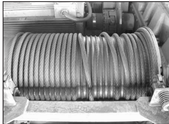
Fig. 135: Steel wire rope and drum damage caused by spooling over the groove flanges.
