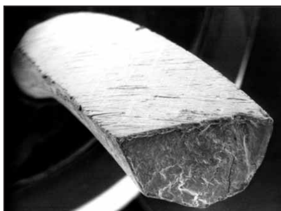
Fig. 21: Severely worn wire with a fatigue break.
