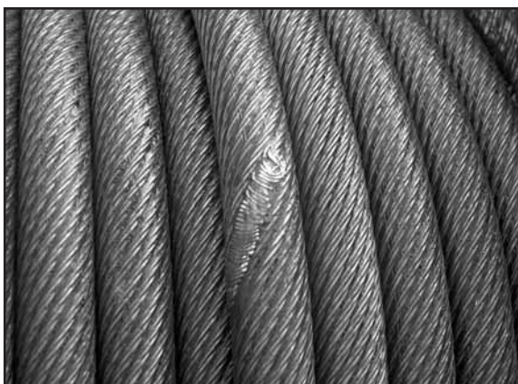
Fig. 144: A strand serving was not removed during rope closing and ended up as an unpleasant decoration of the finished rope.
