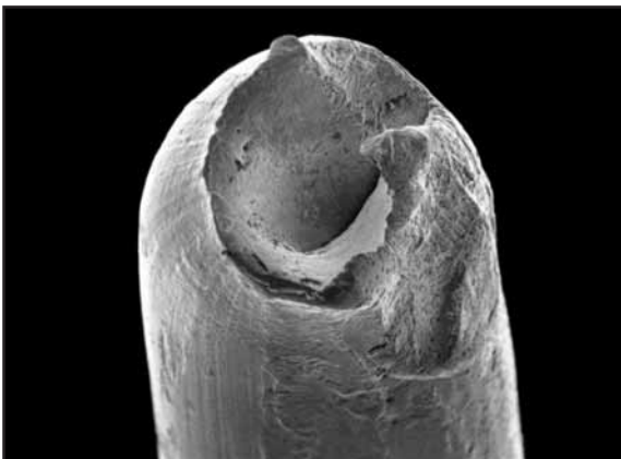
Fig. 39: This locally damaged wire finally failed in tensile overload.
