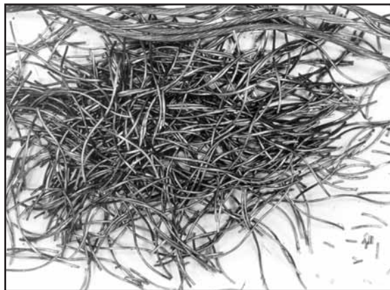
Fig. 85: Opening up this discarded steel wire rope proved that the steel core was no longer in very good condition.
