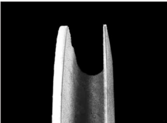
Fig. 122: Severe fleet angles will lead to rope twist and increased wear, both on the wire rope and on the flange of the sheave.
