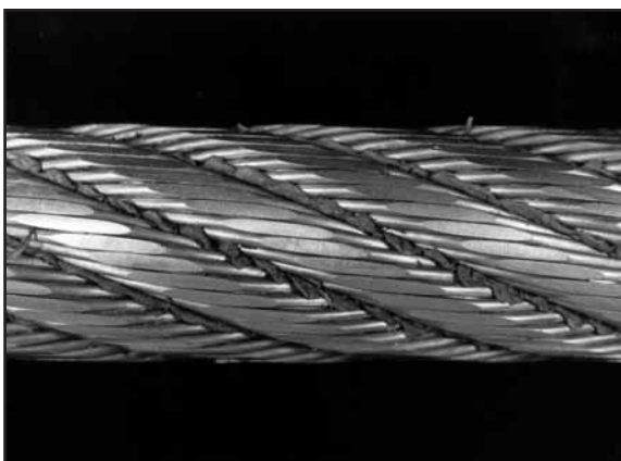
Fig. 4: Regular lay rope with a great amount of uniform mechanical wear. Please note that the rope does not show any fatigue breaks.
