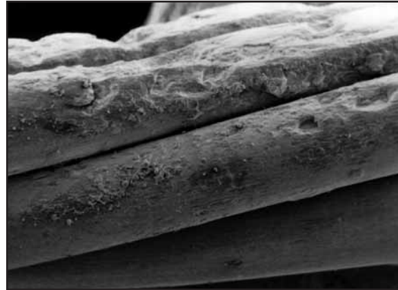
Fig. 29: Pitting corrosion (local corrosive attack creating deep pits).
