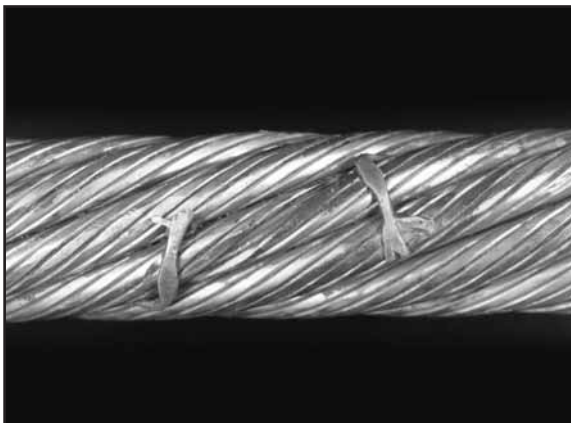
Fig. 116: These two broken wire ends got caught between the wire rope and the sheave causing nicking damage.
