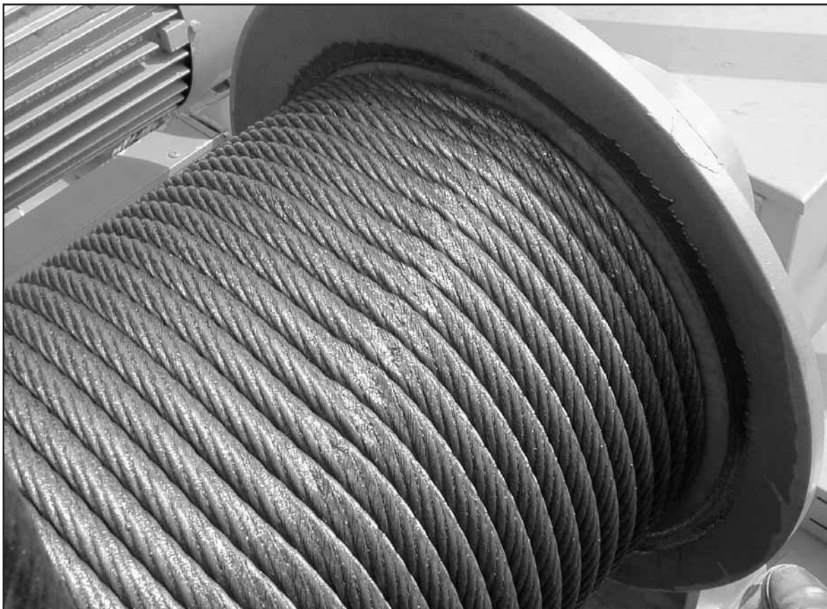
Fig. 124: The inclined wear pattern (cross over zone) shows that the rope is too small for the drum pitch. If it was inclined in the opposite sense, this would be an indication that the rope diameter is too big.
