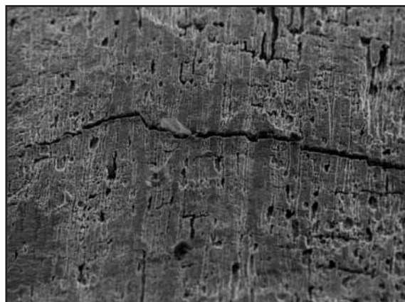
Fig. 14: Pitting and corrosion associated with a fatigue crack (detail of Fig. 13).
