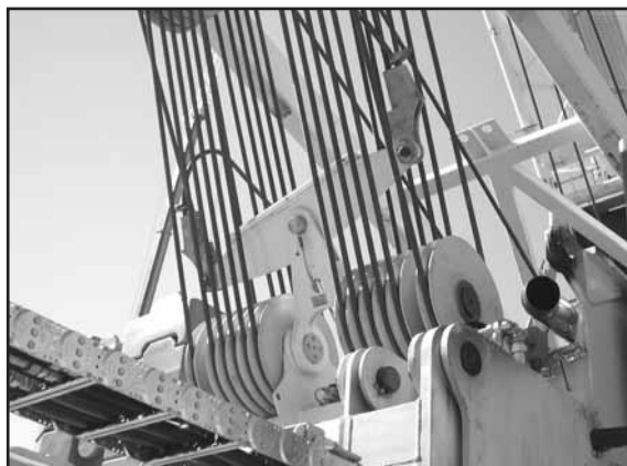
Fig. 147: In multi layer spooling, small diameter differences of two ropes will lead to big differences in the spooled rope lengths (see p. 42).
