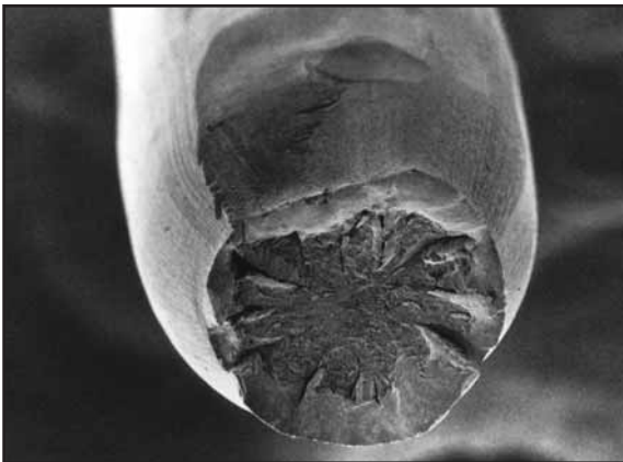
Fig. 37: Cup and cone tensile failure at a crossover point.
