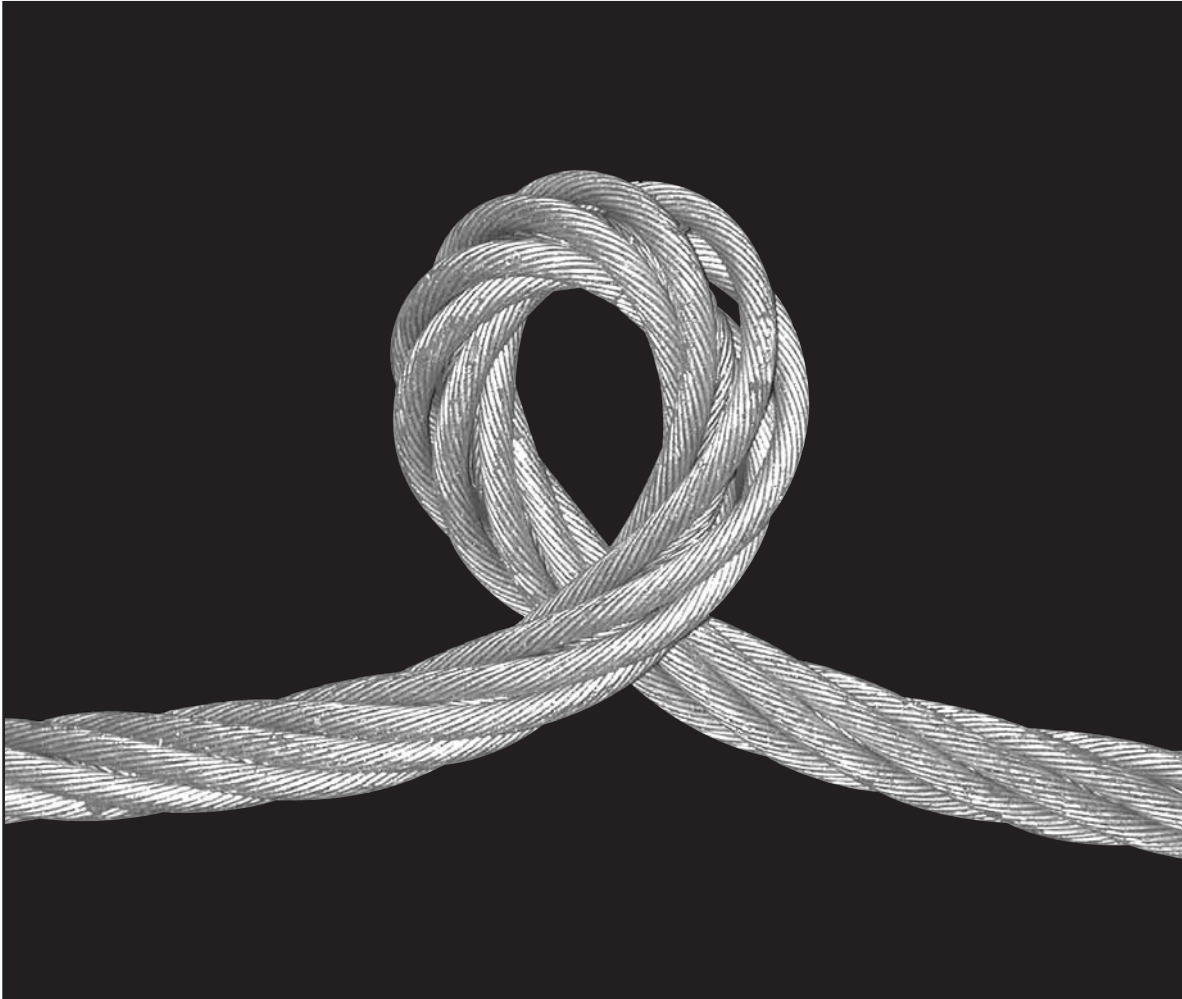
Fig. 104: This rope has been twisted in the opening sense. When slack, it will form a hockle in the closing sense. When hockles are loaded, they might pull tight and permanently deform the rope.
