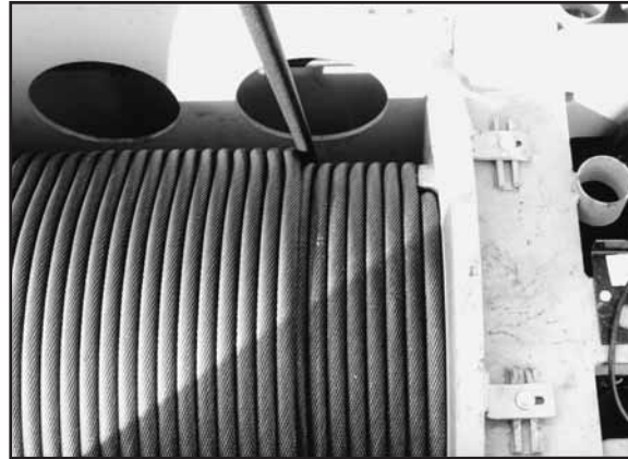
Fig. 126: This rope is spooling onto a multi layer drum with special grooving. The rope is about to cross over one wrap.
