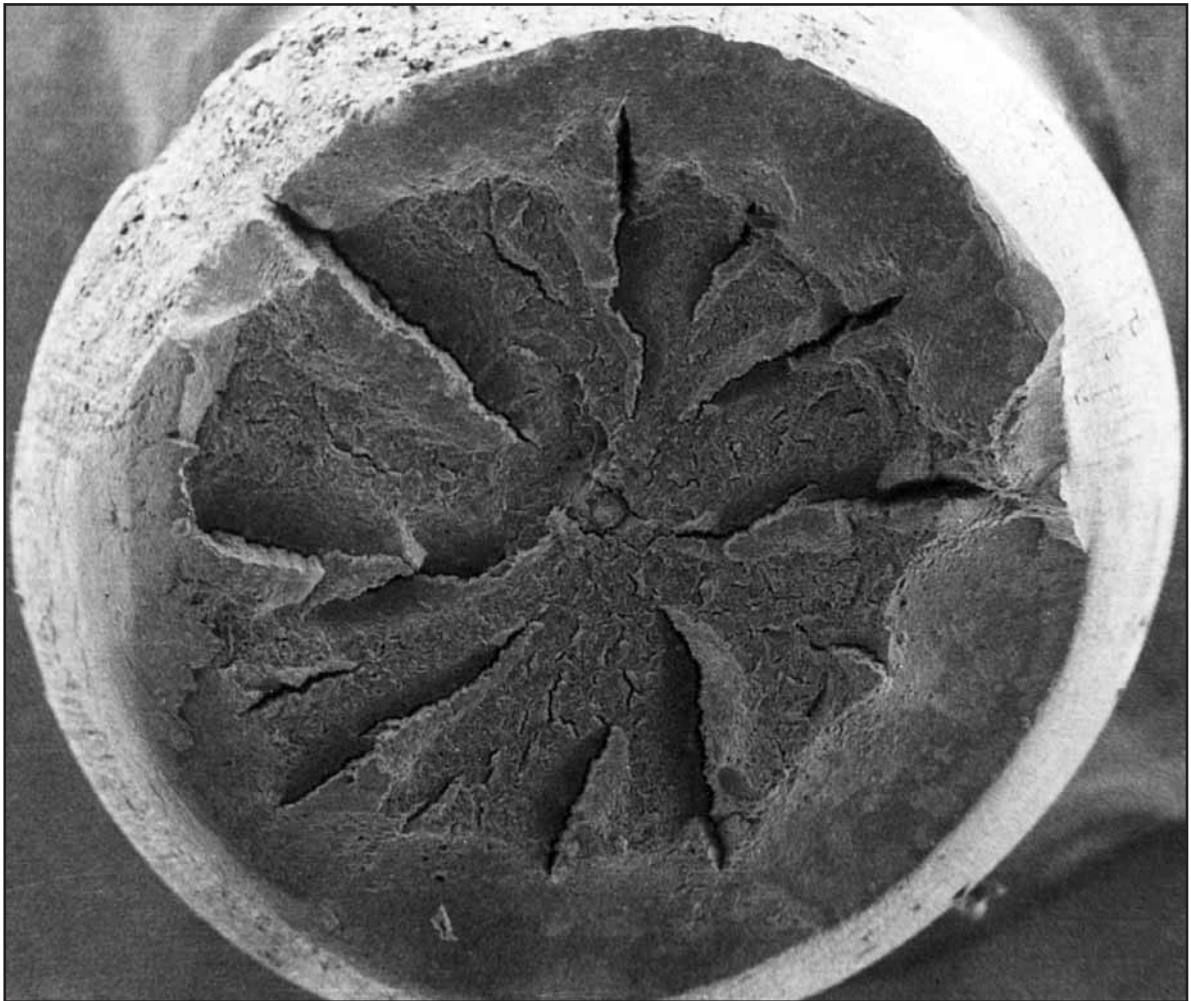
Fig. 41: End view of the cone half of a tensile overload break. The inner cone has failed due to tensile stresses before finally the outer ring fails in shear.
