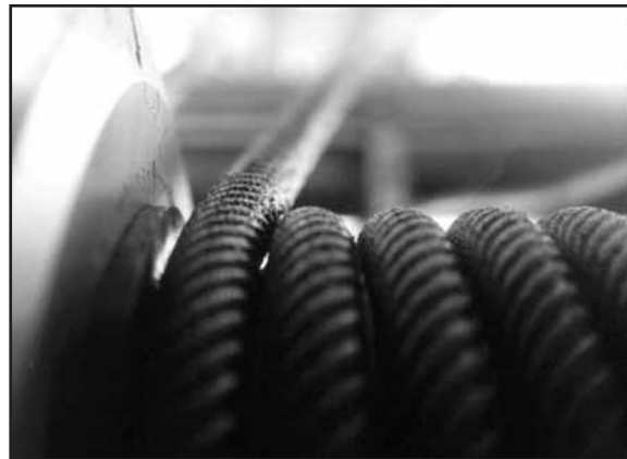
Fig. 128: The fleet angle forces the rope fall entering the drum to rub against its "neighbour", causing severe abrasion and rope twist.
