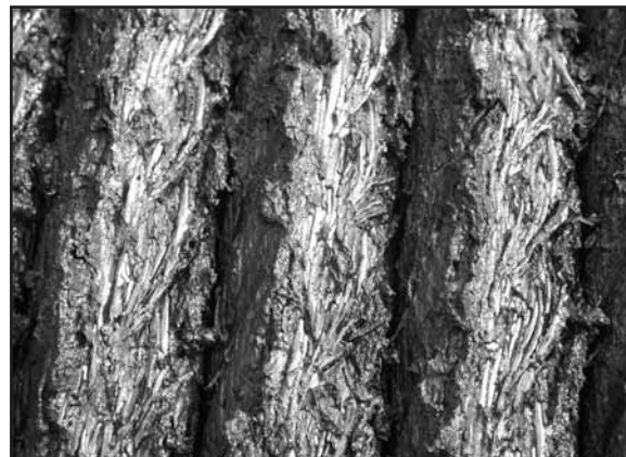
Fig. 137: this rope was ready for discard (see Fig. 136). Further examination showed that every outer wire was broken every 3 cm.
