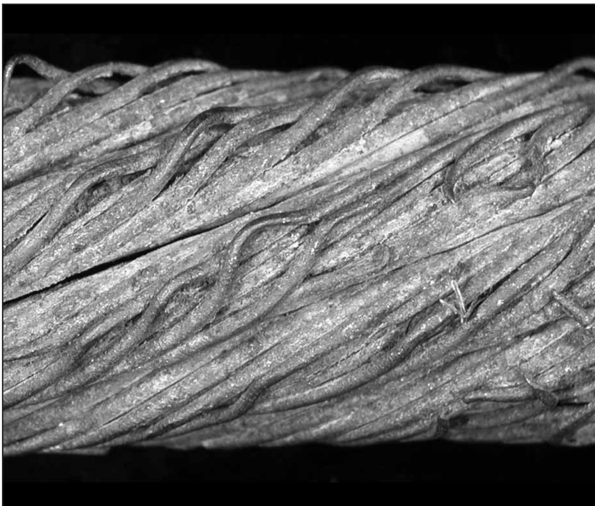
Fig. 80: This hoist rope from a ladle crane has been exposed to elevated temperatures for too long. As a result of this the outer wires have annealed, softened and then lengthened in service.
