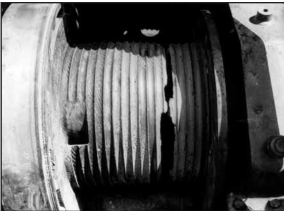
Fig. 134: If the load is always picked up at the same location, always the same sections on the drum and on the rope will be worn.
