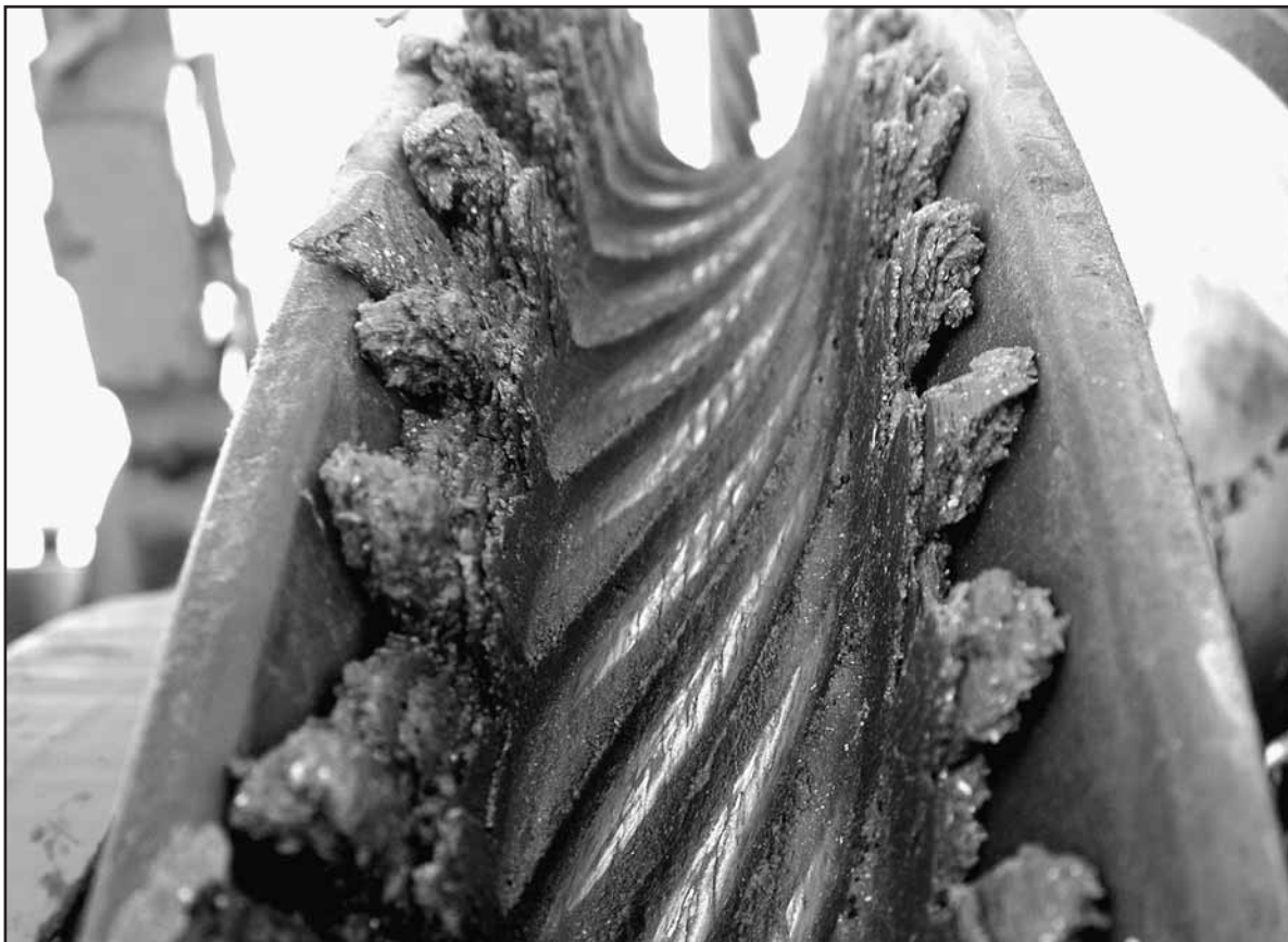
Fig. 118: Lubricant deposition at regular intervals on the flanges of a sheave as opposed to a continuous coating often indicate the formation of negative imprints.
