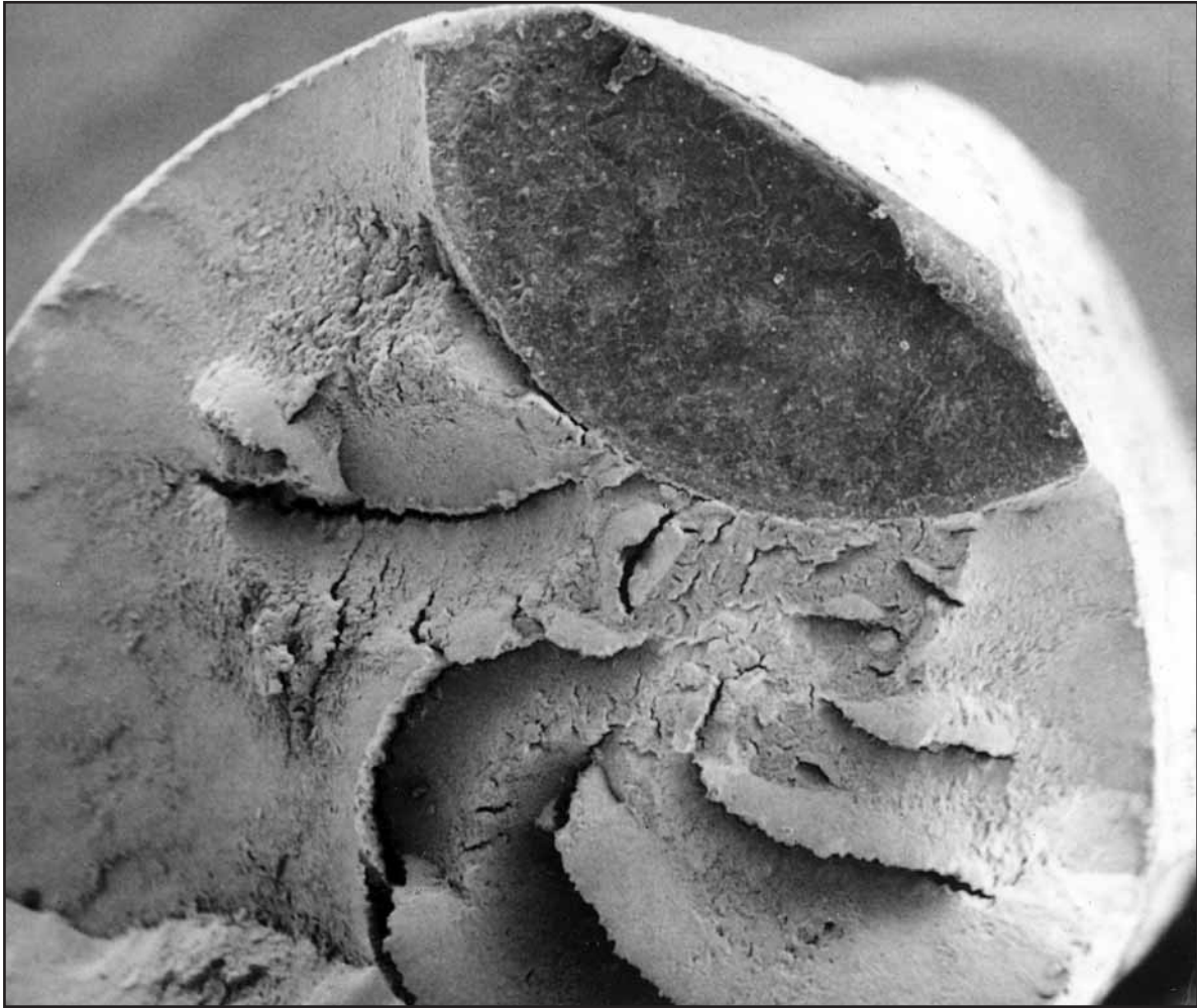
Fig. 15: A fatigue crack starting at the point of contact with a sheave. Obviously the crack propagated concentric to its point of initiation. The crack only became visible after destroying the strand in a pull test.
