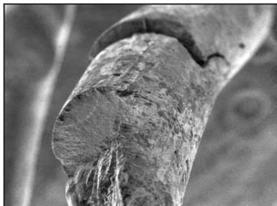
Fig. 23: Two adjacent fatigue cracks. This kind of failure can often be seen if wires are subjected to local bending and compression.
