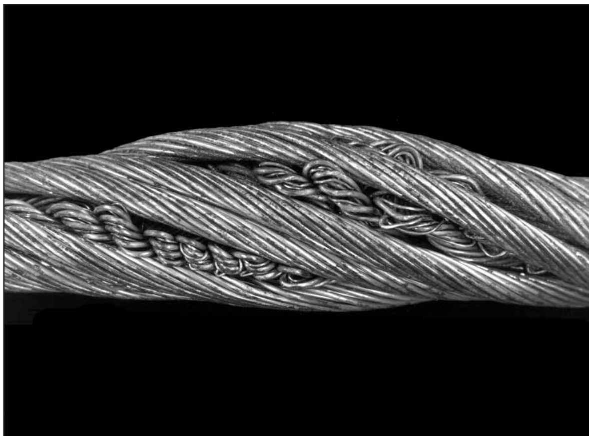
Fig. 97: A surplus of strand lengths in the steel core caused by twisting the rope has been accumulated at one point by a sheave. Defects like this are usually found at the end of the motion of the sheave over the rope (or of the rope over the sheave).
