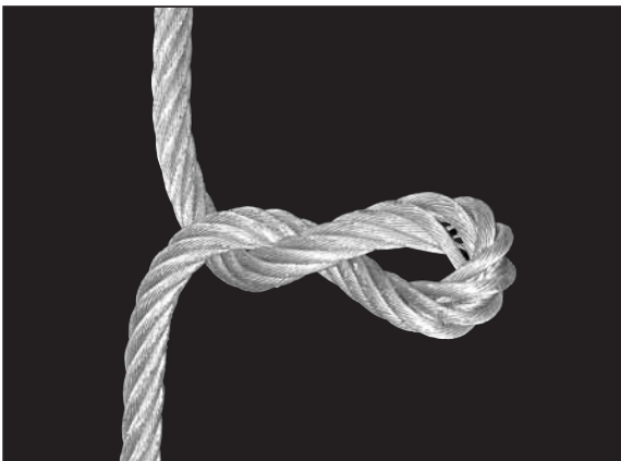
Fig. 105: This rope has been twisted in the closing sense. When slack, it will form a hockle in the opening sense.
