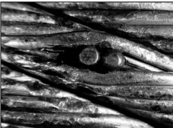
Fig. 59: Damage caused by shot-blasting a crane before repainting. Shot stuck to the lubricant and later wedged into the strand.
