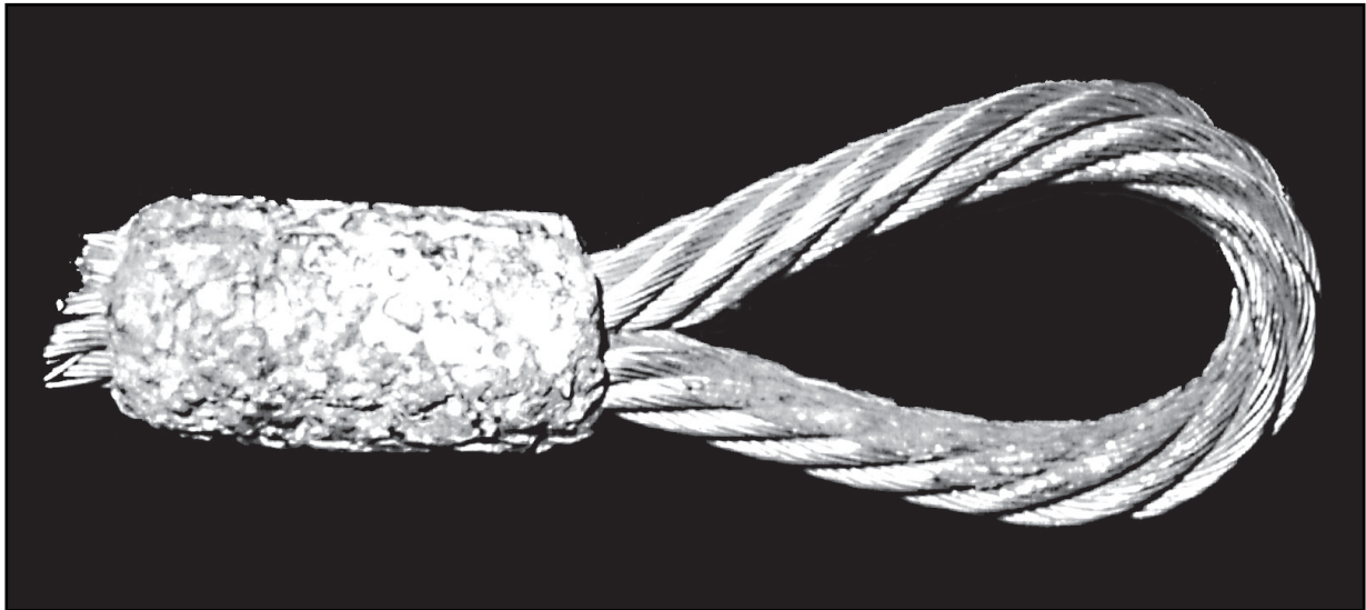
Fig. 51: Corroded aluminium clamp
