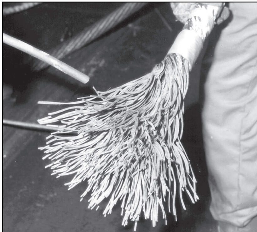
Fig. 69: Drying the rope brush
