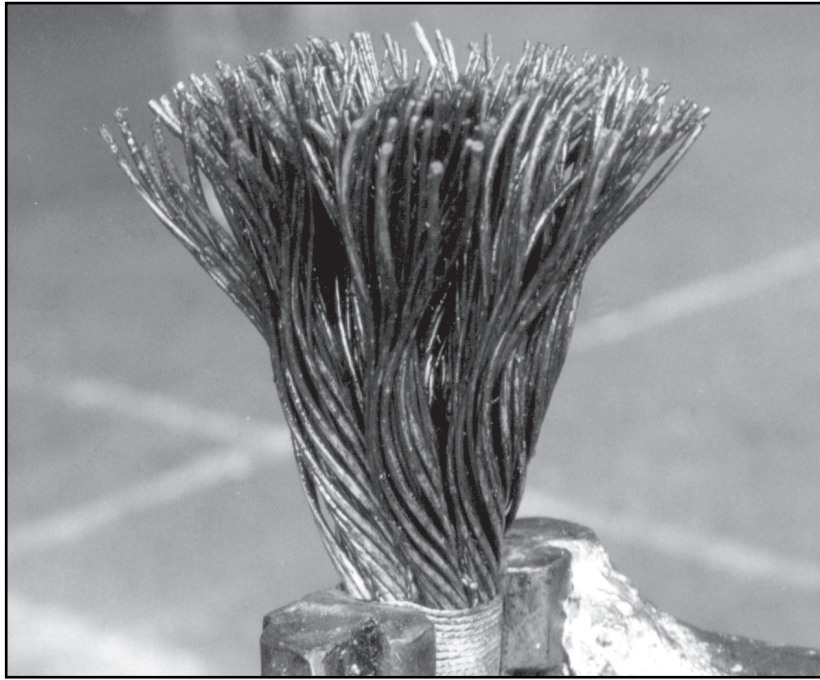
Fig. 68: Broom formed for socketing by unlaying the strands
