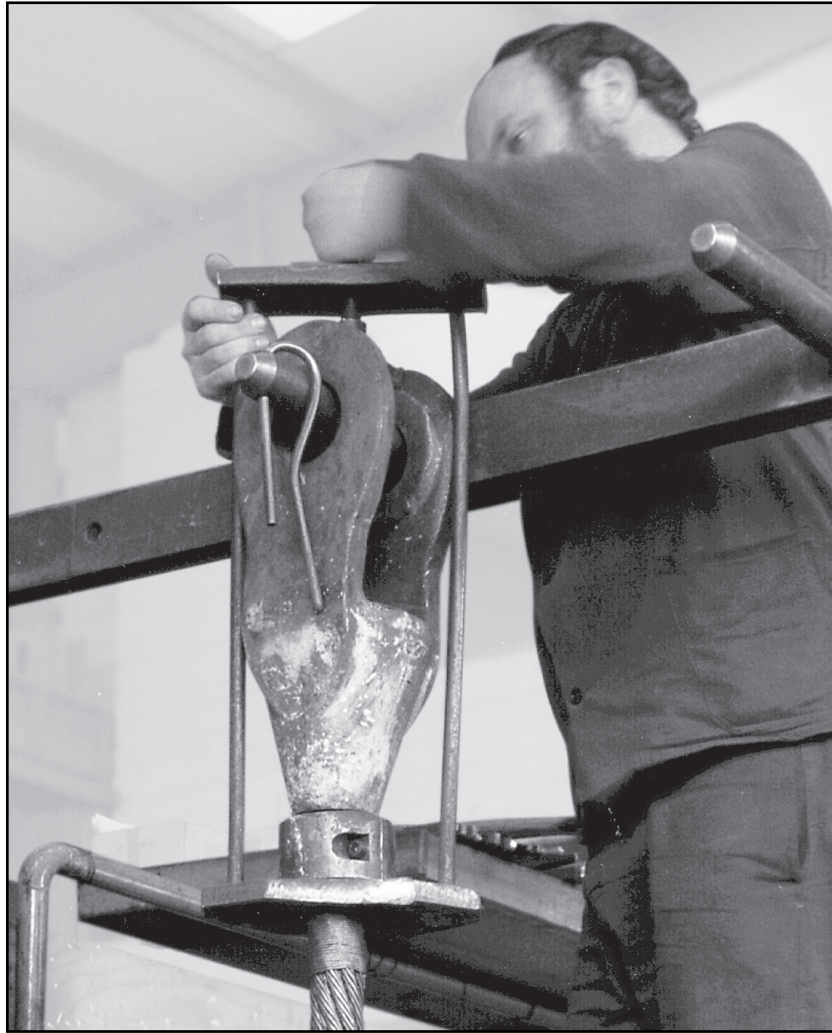
Fig. 70: Adjusting the wire rope socket
