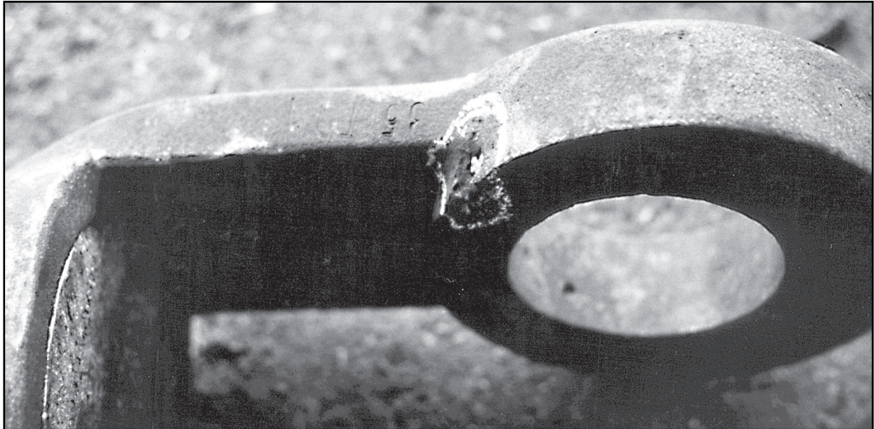
Fig. 67: Casting defect on an open wire rope socket
