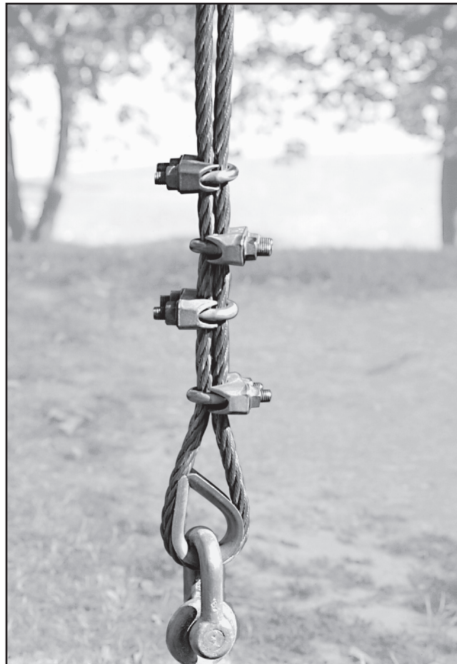
Fig. 8: Rope end connection with wire rope clips fitted incorrectly
