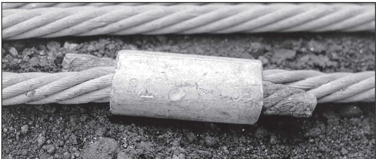
Fig. 49: Incorrect connection of two ropes
