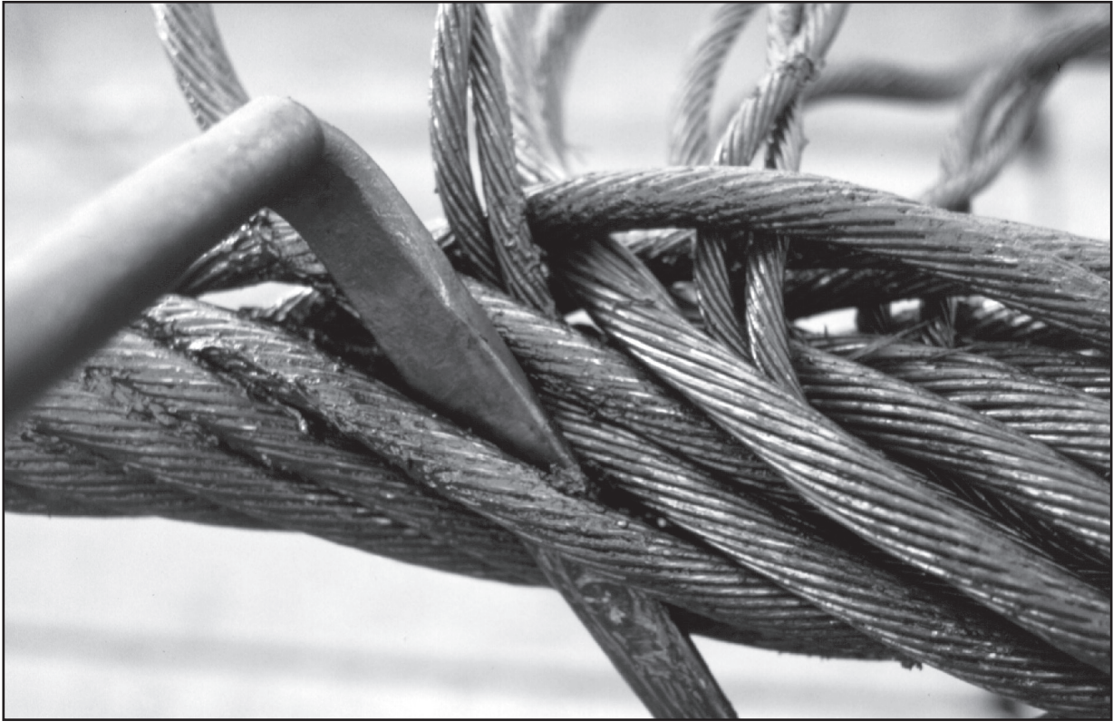
Fig. 33: Splice on an eight-strand wire rope with a steel core (detail)
