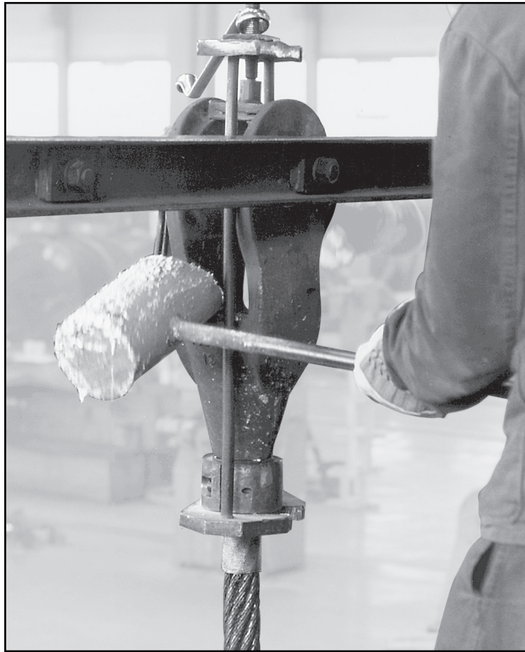
Fig. 74: Slow pouring of the spelter material
