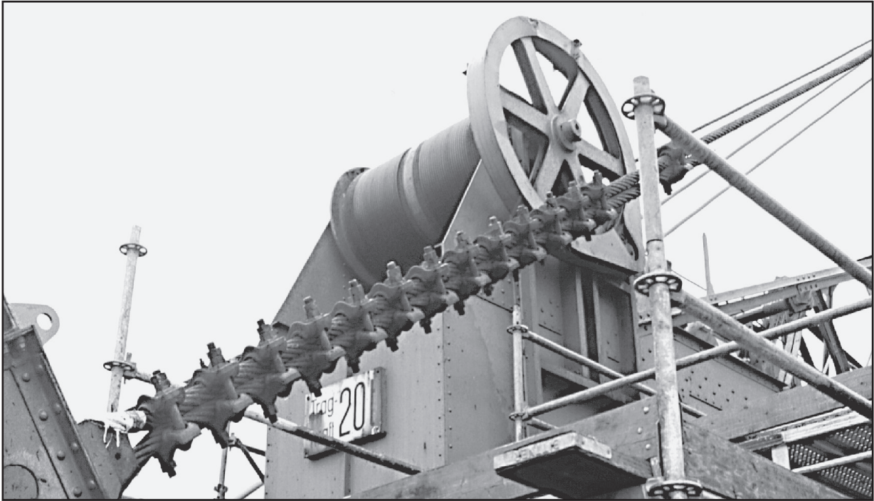
Fig. 12: Rope end connection fitted with wire rope clips for mining applications.
