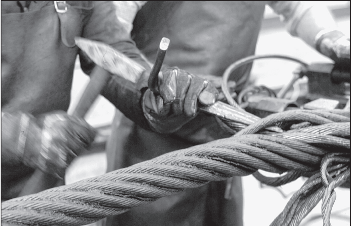
Fig. 31: Hammering in the marlin spike in
