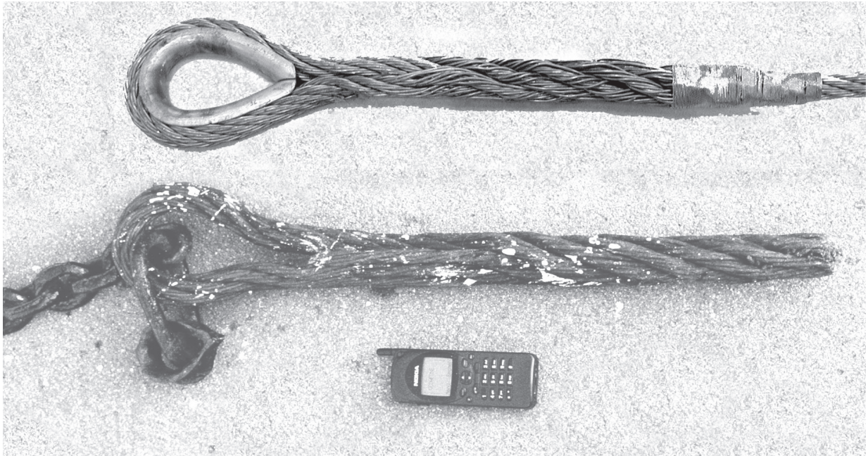
Fig. 15: Comparison of the Great Britain splice discovered at Bristol (bottom) and the replica made during this study (top)
