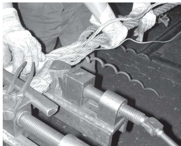
Fig. 10: Wrapping of the first wire of the dead end of strand number 1 around the live part of strand number 1
