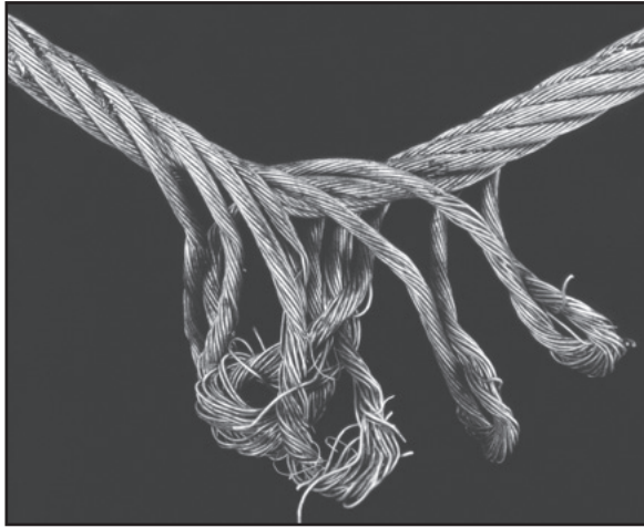
Fig. 39: Surplus length of the outer strands caused by unlaying the rope
