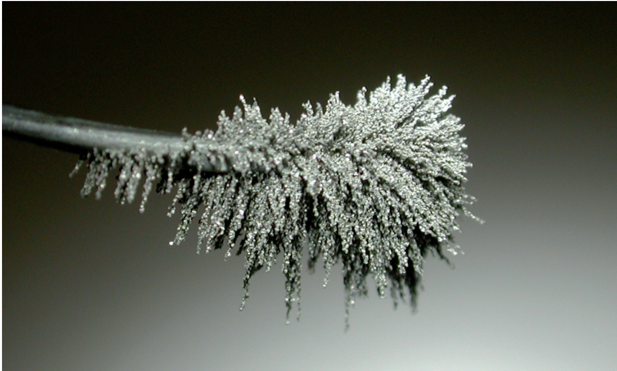
Fig. 4: The wire fracture end of wire which has failed due to tension- tension fatigue after dipping it into iron powder. The wire is highly magnetic.
