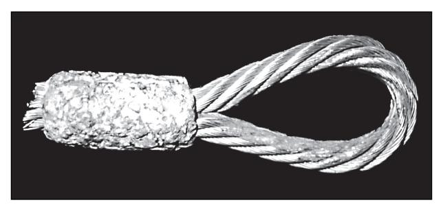
Fig. 51: Manchon aluminium corrodé
