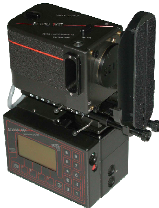
Figure 10: Round shot camera with a slit aperture to produce a continuous image.
