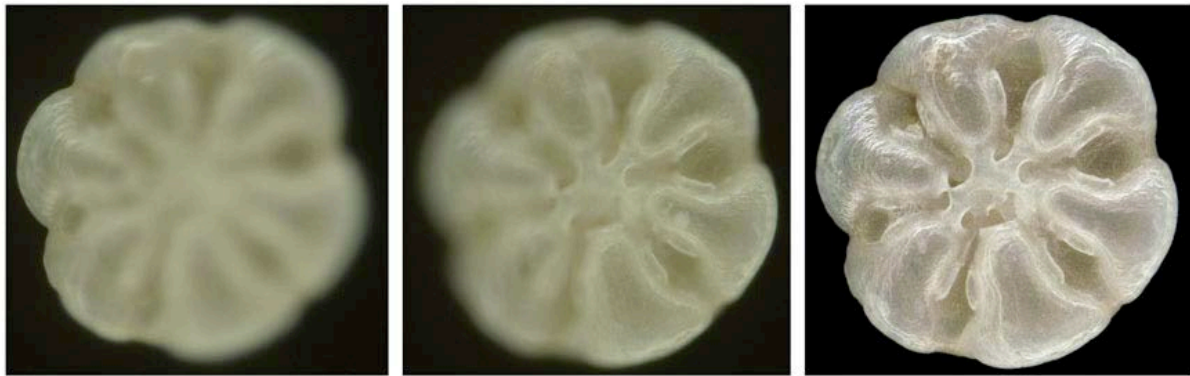
Figure 17: First (left) and last (middle) photo of a series of 27 photographs and the stacked and “Photoshopped” resulting image (right)
