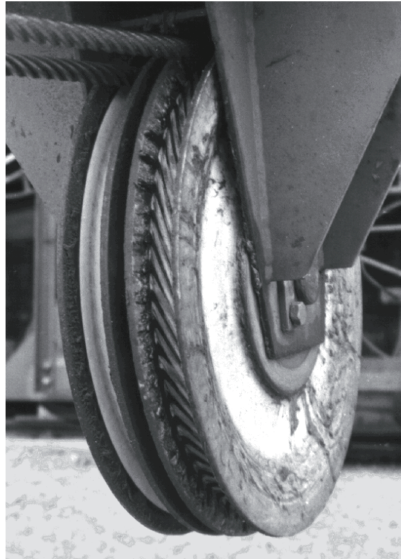
Fig. 1: Wire rope sheave with negative impressions
